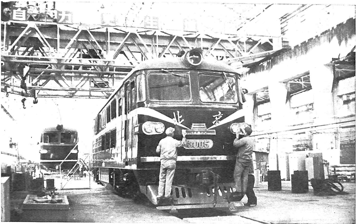
Putting the finishing touches on a 3,000-horsepower diesel locomotive at the "February 7" plant.
